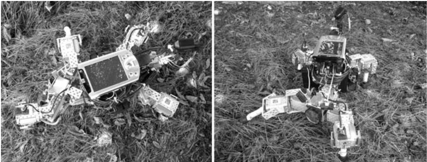
Fig. A.1. The physical four-legged walking machine AMOS-WD02. Left: Top view while turning its backbone joint. Right: Front view while in its standing position
