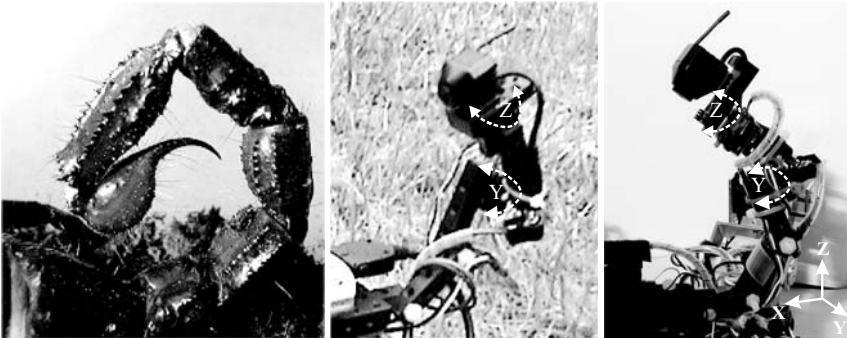
Fig. 4.15. Left: A scorpion's tail with a sting (modified from S.R. Petersen 2005 [160] with permission). Middle: The tail of the four-legged walking machine AMOS-WD02. Right: The tail of the six-legged walking machine AMOS-WD06. The two DOF tail is constructed in an abstract form of a scorpion's tail. It is mainly used to install the camera
